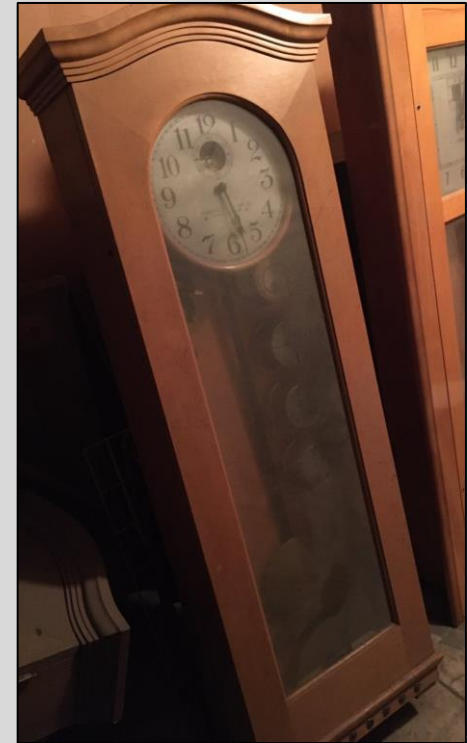
Two, Standard Electric Time Control clocks from the Eliot Elementary Schools. Used as the master clock for controlling alarm bells. Wood case with door. Wall mounted. #'s 3841 A & 3841 B
