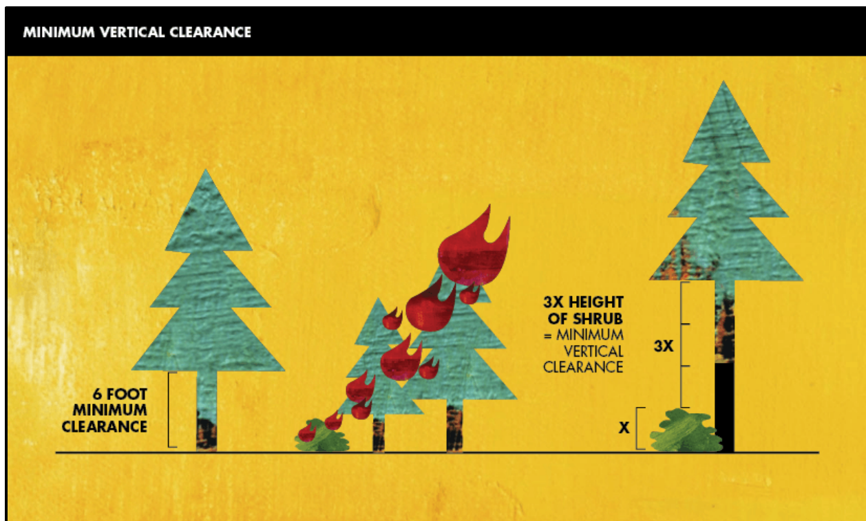
Figure F.4. Minimum vertical clearance.
